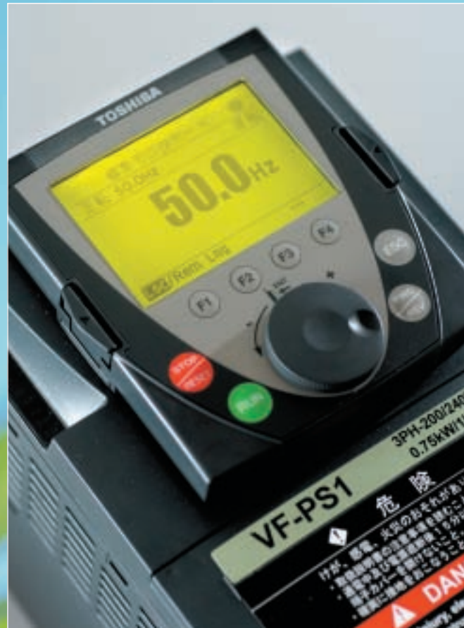
Photo is PS1 with LCD remote keypad option.
