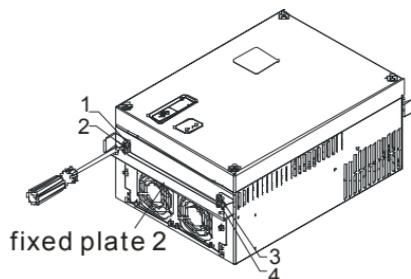
Step 3: Please notice that it doesn't need to put those 8 screws shown in the following figures back to the drive. Moreover, please make sure that these 2 different fixed plates are put in the correct side as shown in the figures.
