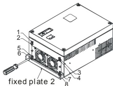
Step 2: place the 8 screws back in to secure the fixed plate 1 and fixed plate 2 (as shown in the following figures) with the following torque.
