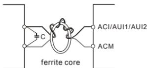
**wind each wires 3 times or more around the core**
