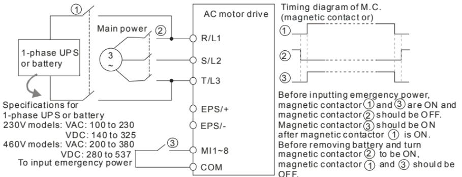
Figure 4 Apply to two batteries with main battery voltage is lower than 280Vdc
