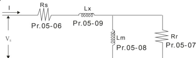
Equivalent circuit for VFD-VL series
