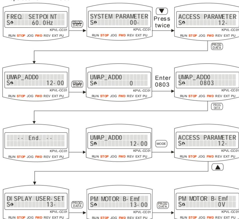
Example 2: If it needs to enter parameter address 2102H and 211BH by the digital keypad, 211BH needs to be converted to binary value before entering.
