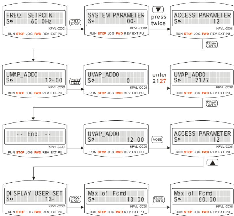
In the following, it shows the factory setting of Pr.12-00 to Pr.12-29. You can change the setting as required.
