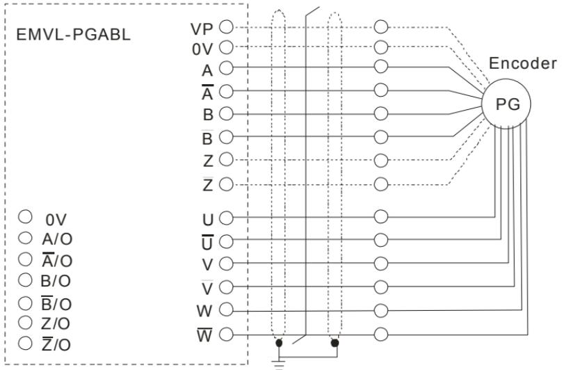
4. Output Signal Setting of the Frequency Divider
