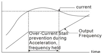
actual acceleration time when over-current stall prevention is enabled
