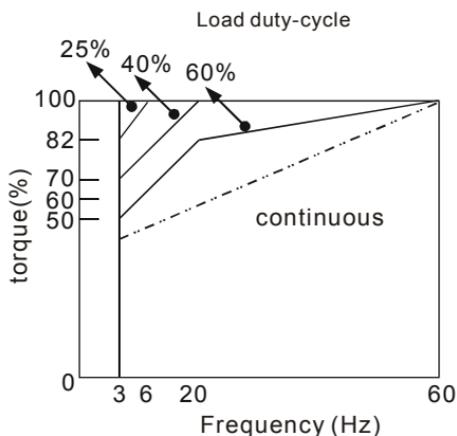
5. If 100% continuous torque is required at low speed, it may be necessary to use a special inverter duty motor.
