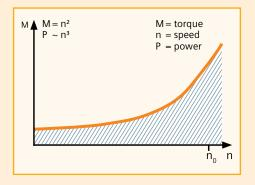
**Low Overload (LO)** is generally used for applications demanding a low level of dynamic performance (continuous duty), square-law torque characteristic with low breakaway torque and low speed precision.
