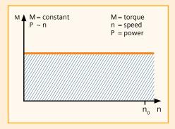
**High Overload (HO)** is generally used for applications demanding a higher dynamic performance (cyclic duty), as well as constant torque characteristics with a high breakaway torque.
