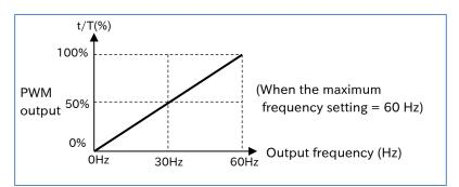
(Example 2) PWM output for output current monitor ([C027] = "Output current (01)")
