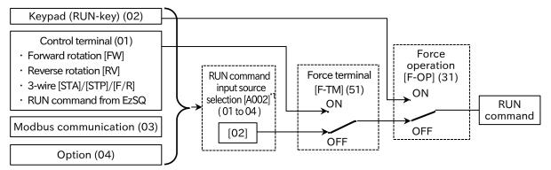
(The values in square brackets and the switch positions shown in the figure are the default values. In addition, all functions not assigned to input terminals [1] to [7] are turned off.)
