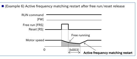
If restart after reset release is set to active frequency matching restart, power-up startup also operates in active frequency mathing.
