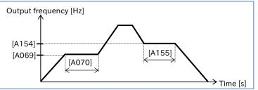
Applying the hold function using the [HLD] input terminal
