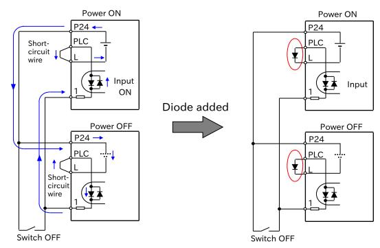
If there is no diode, the current will flow round and the input will turn on even though the switch is off. Diodes are installed instead of the short-circuit wires to prevent current flow round.
