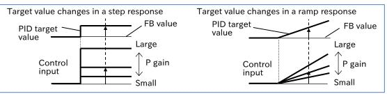
(2) I-operation: Operation in which the deviation is integrated per unit time and added to the control input. In a P-operation, changes in output are reduced as the PID target value and FB value get closer, increasing the time required to reach the target value, which is compensated for by the I-operation.
