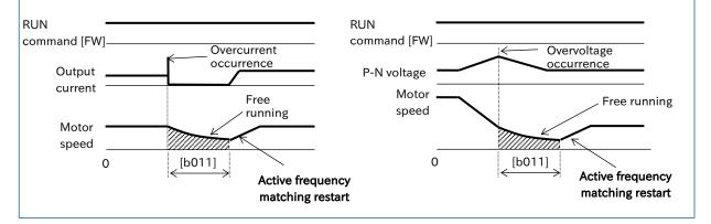
• Even when the retry operation is selected for a trip, if the trip factor has not been released after the retry wait time, the trip is detected again. In this case, increase the retry wait time.
