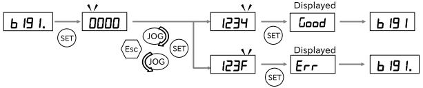
(2) If the password is correct, "Good" is displayed and [b031]/[b037] can be changed. If the password is incorrect, "Err" is displayed and the inverter returns to the original state (password lock state). After turning on the power again or about 10 minutes pass without any key operation, the password lock state is automatically activated.
