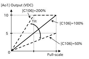
(Example 2) When the output current 0 to 100% is the output of 0 to 10 VDC
