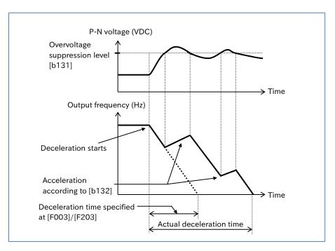
• If the "Overvoltage suppression active time [b132]" is shortened, an increase in the output frequency due to acceleration is greater than that of the deceleration, and as a result, the motor may not be able to stop. In such a case, increase the "Overvoltage suppression active level [b131]".
