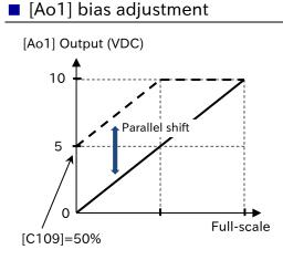
(Example 1) When the output frequency from 0 to the maximum frequency is the output of 0 to 5 VDC
