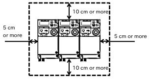
\* Even in case WJ-C1 and WJ200 series are installed together, leave enough clearance around them as shown on the left. Also, follow the current derating of each model.
