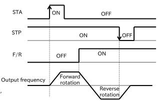
This example shows a terminal assignment consisting of Terminal 1 = [STA], Terminal 2 = [STP], and Terminal 3 = [F/R].
