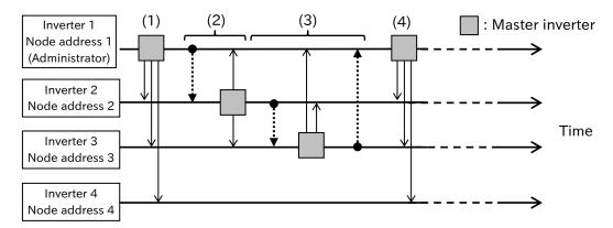
(1) When EzCOM communication starts, the inverter specified by the administrator inverter becomes "Master inverter". In the above example, inverter 1 = administrator inverter = the latest master inverter.
