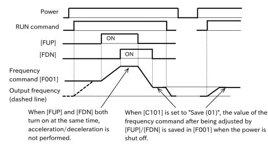
Remote control speed data clearing [UDC] operation
