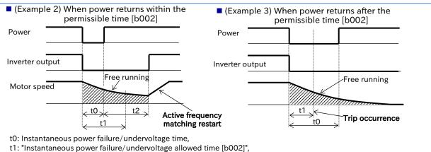
t2: "Retry wait time after instantaneous power failure/undervoltage error [b005]"
