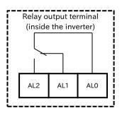
\* The function assigned to the relay output terminals when shipped from the factory/initialized is "Alarm [AL]".
