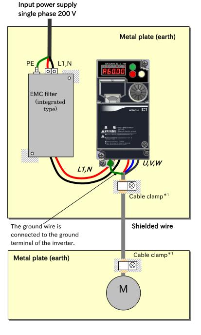
The filter is integrated and mounted between the inverter and the metal plate. Remove paint from the ground terminal, ensure sufficient contact area, and ground. ( ///// part in the figure left)
