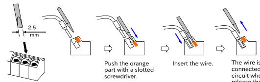
The wire is connected to the circuit when release the slotted screwdriver.
