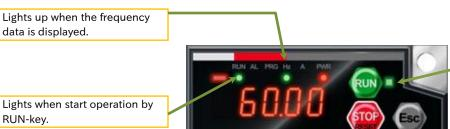
When RUN command source is keypad, the RUN-key is enabled and the RUN command indicator LED lights.
