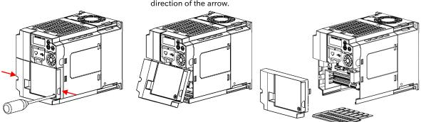
While pressing in the direction of the arrow, remove the terminal block cover from below.
