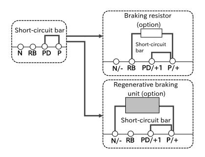
Cautions for the brake resistor connection terminals ([P/+], [RB]) and regenerative brake unit connection terminals ([P/+], [N/-])
