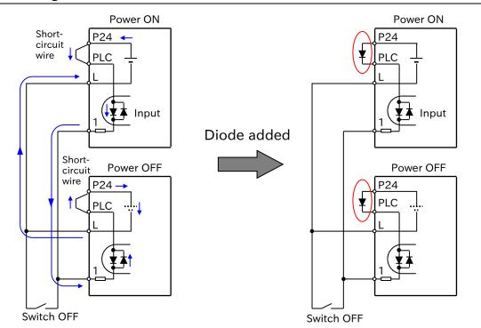
If there is no diode, the current will flow round and the input will turn on even though the switch is off.
