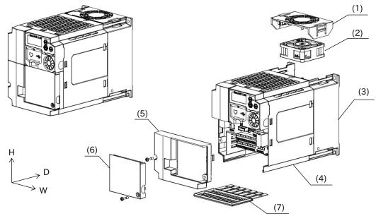
\* The W and H dimensions are the same, but the D dimensions differ depending on the model due to the difference of the cooling fin.
