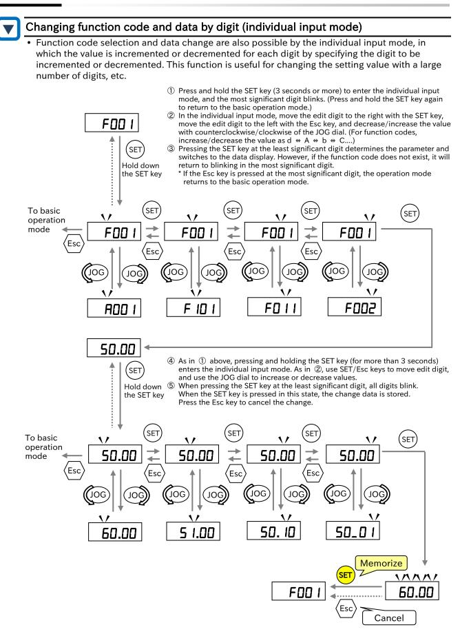
• The individual input mode is valid for the function code and numeric data parameters. It is invalid when the setting range is a number selection such as 01, 02, 03....
