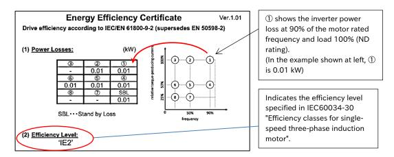
(4) The inverter losses at each point shown by the numbers on the Output Frequency vs. Load Factor (ND Rating) graph at the right of the figure above are shown in the table on the left.
