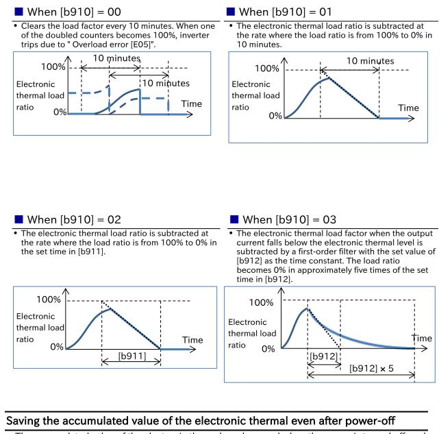
• The accumulated value of the electronic thermal can be saved when the power is turned off, and can be read the next time the power is turned on.
