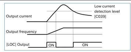
When [C038] is set to "Enabled only during constant speed (01)"
