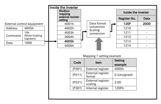
• The external address 4005h is mapped to the inverter internal register 120Fh, and the external data 1000d is written.
