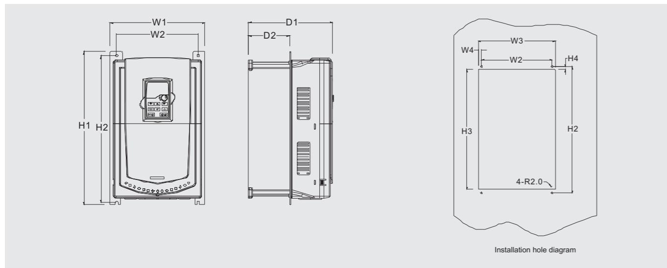
■ Floor installation diagram for inverters of 380V 220 ~ 315kW(660V 250 ~ 350kW)
