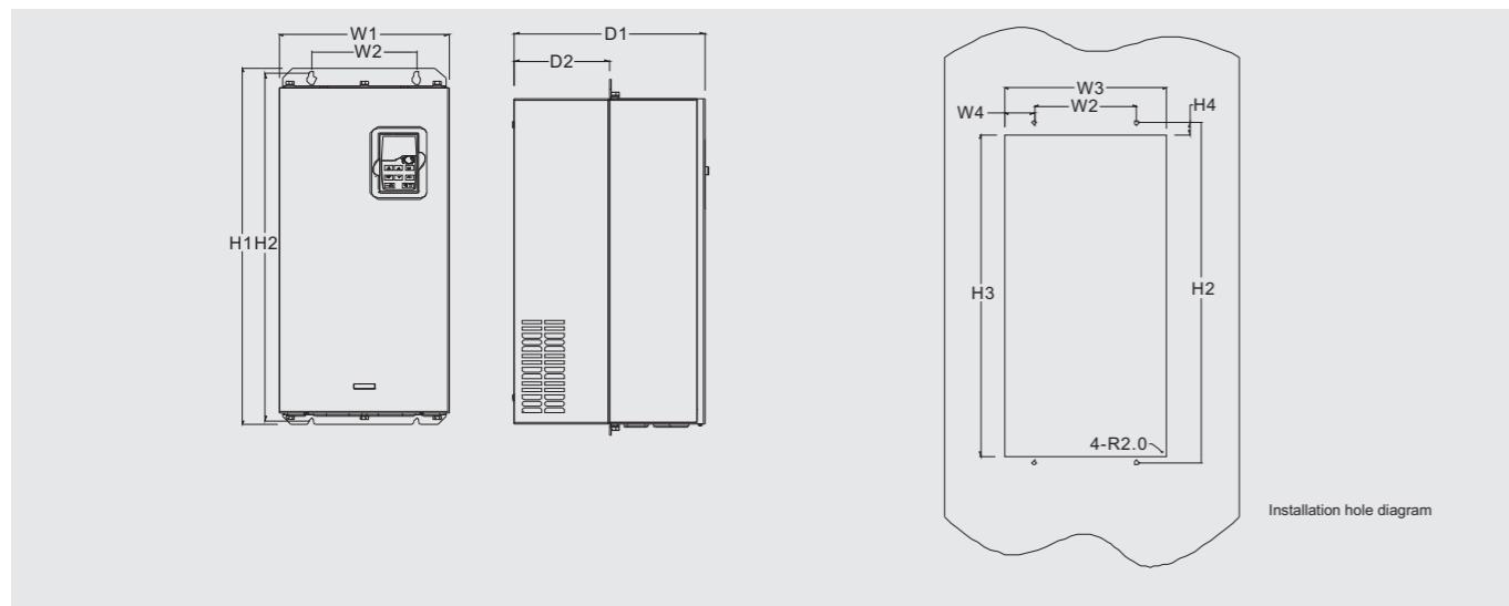
■ Floor installation diagram for inverters of 380V 350 ~ 500kW(660V 400 ~ 630kW)
