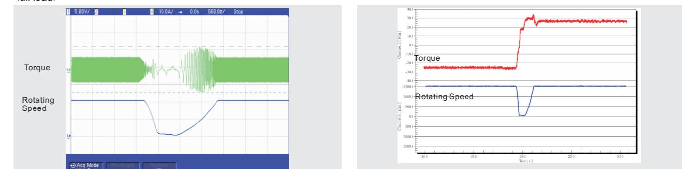
The FWD/REV current, torque and rotating speed waveforms in synchronous motor torque control mode with 100Hz running frequency and full load.
