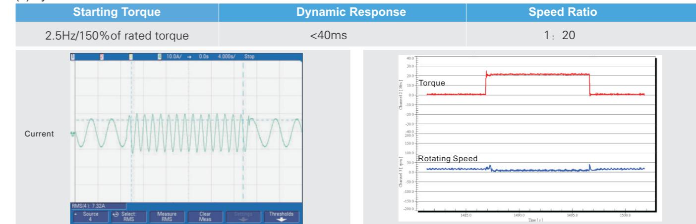
The current, torque and rotating speed waveforms when sudden loading or unloading in asynchronous motor open loop vector control mode with 0.25Hz running frequency and full load.
