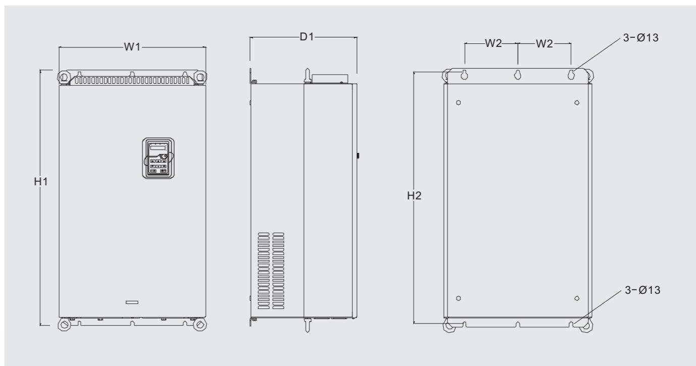
■ Wall installation diagram for inverters of 380V 220~315kW(660V 250~350kW)
