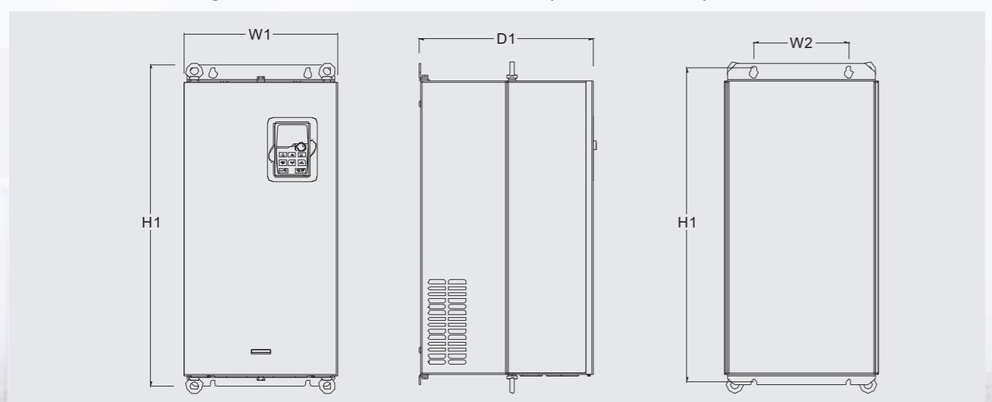
■ Wall installation diagram for inverters of 380V 132~200kW(660V 160~220kW)
