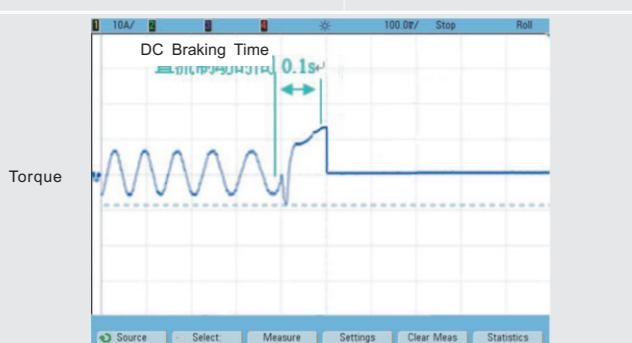
The current waveform in asynchronous motor SVPWM control mode with 100% braking current when the starting frequency is 10Hz and the braking time is 0.1s.
