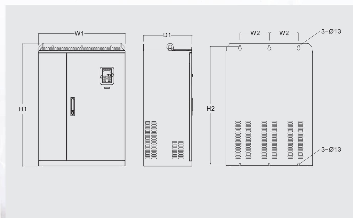
■ Flange installation diagram for inverters of 380V 1.5 ~ 30kW
