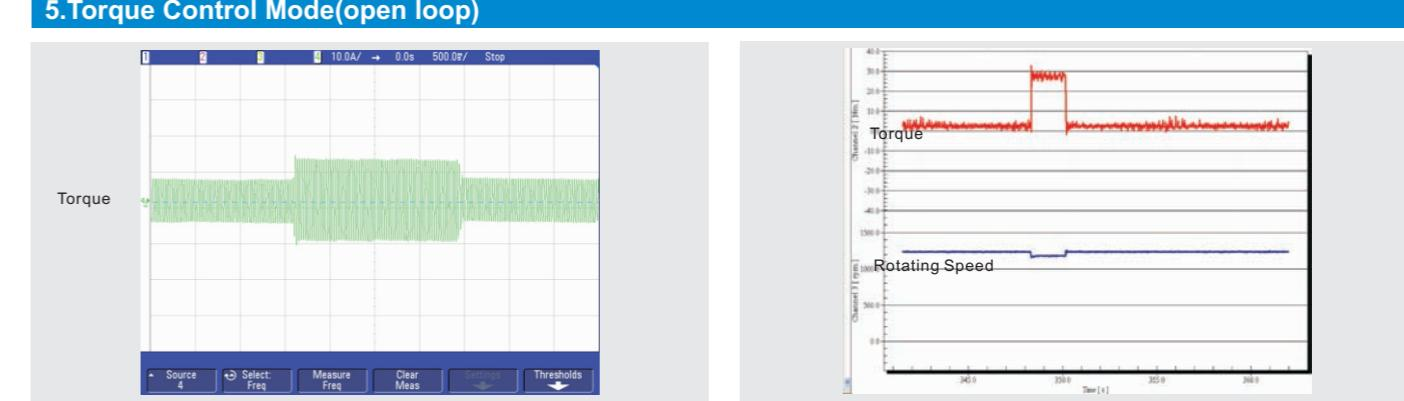
The current, torque and rotating speed waveforms when sudden loading or unloading in asynchronous motor torque control mode with full load.
