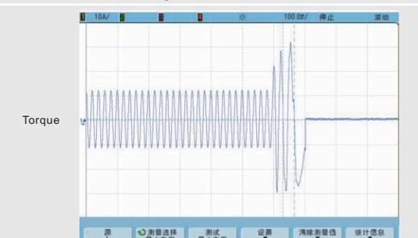
Flux braking current waveform when the running frequency is 50Hz, deceleration time is 0.1s with full load in asynchronous motor SVPWM control mode
