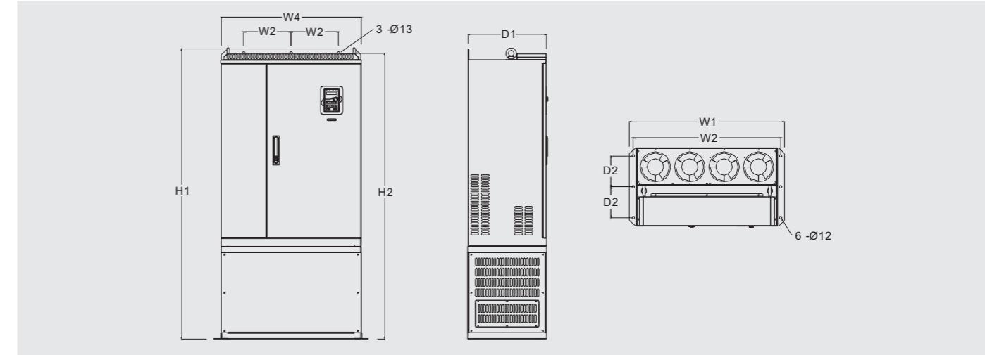
■ Flange installation diagram for inverters of 380V 37 ~ 110kW(660V 22 ~ 132kW)
