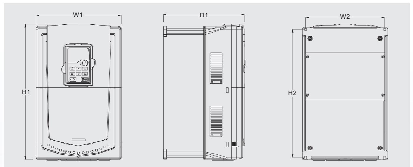
■ Wall installation diagram for inverters of 380V 37~110kW(660V 22~132kW)
