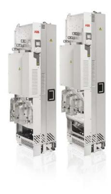
ACS580-04 drive modules with IP00 protection class extend the power range from 250 to 500 kW, and voltage range from 380 to 480 V. The modules are available in frame sizes R10 and R11.
