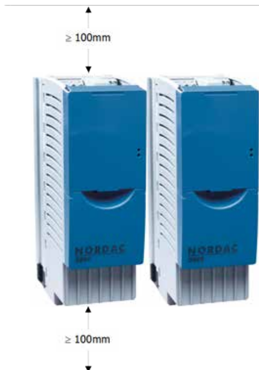
Fig. 3 Mounting distances for SK 5xxE
