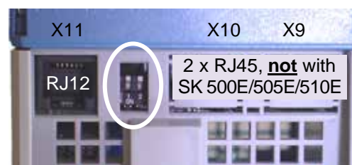
Fig. 11 Top side of FI with RJ12 / RJ45 connection
