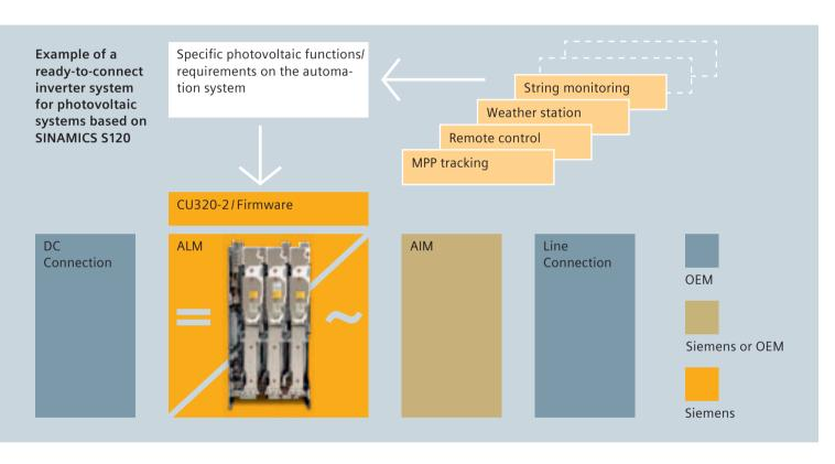
SINAMICS S120 Active Line Modules and Active Interface Modules, as core components of the ready-to-connect inverter, are available in different power stages depending on the particular application.
