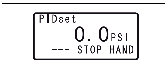
Fig. 6-227: How PID set value is displayed when unit setting is "PSI" (Pr. 759 = "4")
