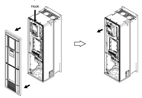
Figure 5.7 Removing the Keypad
