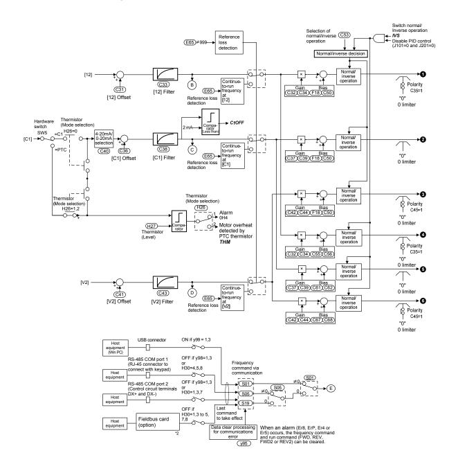
Figure 7.1 (1) Frequency Command Block
