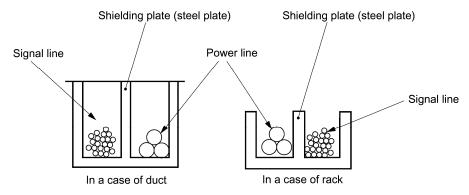
Figure A.7 Separate Wiring
