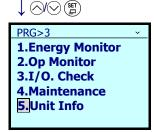
3. Use the ⊘/ ⊗ keys to select [4. Maintenance], and confirm with the (♣) key.
