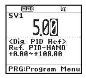
Figure 5.15 Setting the PID Process Command (display sample)
