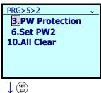
3. "3. PW Protection" indicates that password protection is off (function codes can be revised). To turn password protection on (function codes cannot be revised), select "3. PW Protection" and confirm with the (st) key.
