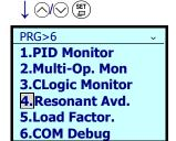
7. Using the key to move the cursor to Fjmp3 and pressing the key at the next point of resonance sets resonance prevention point 3 (Fjmp3).
