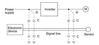
Figure A.5 Electrostatic Induced Noise
