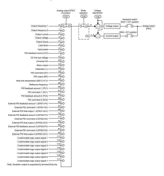
Figure 7.6 Terminal [FM1] Output Selector
