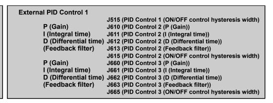
The table below lists function codes to be used for setting the P (gain), I (integral time), D (differential time) and feedback filter for external PID controls.
