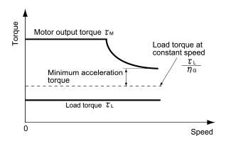
Figure 3.4 Example Study of Minimum Acceleration Torque
