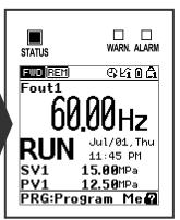
Light alarm (factor exists)Light alarm release reservation (factor exists) Released (normal display)
