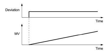
■ D differential time (PID control 1: J112 / PID control 2: J212)
