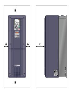
Figure 5.1 Mounting Direction and Required Clearances
