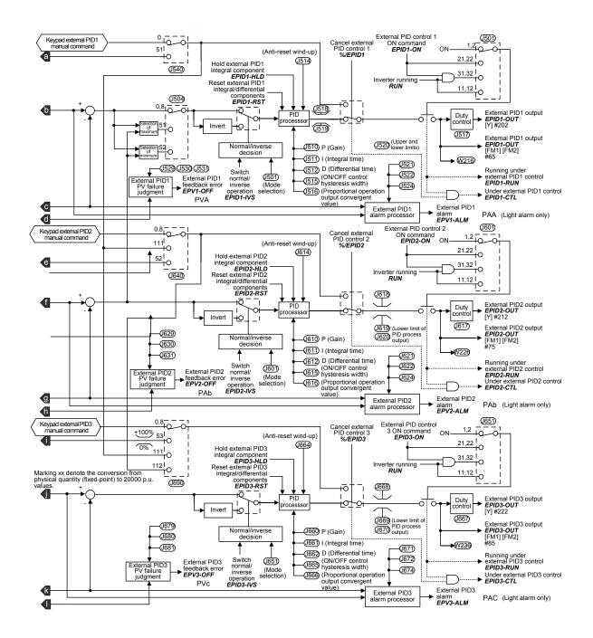
Figure 7.5 (2) External PID Process Control Block
