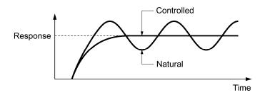
■ Feedback filter (PID control 1: J113 / PID control 2: J213)
