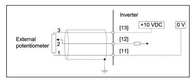
Figure 4.9 Dimensions of External Frequency Command Potentiometer and Connection Example
