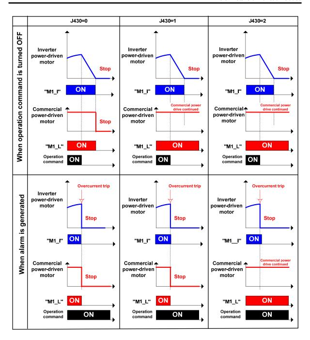
Commercial power-driven motors (including forced on motor) can be stopped in the following methods.
