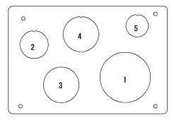
For instructions on how to punch out semi-perforated sections in the wiring plate and set conduits on the wiring plate, refer to Chapter 5, Section 5.1.2.1 "(2) Punching out semi-perforated sections in the wiring plate and setting cable glands or conduits."
