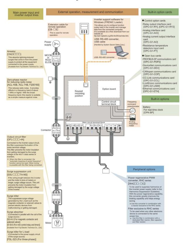
Figure 4.1 Configuration Example
