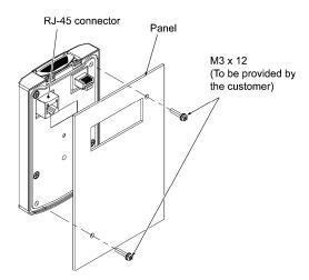
Figure 5.9 Mounting the Keypad
