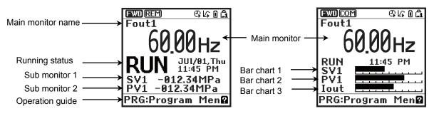
The display type can be selected easily in Programming mode as follows.
