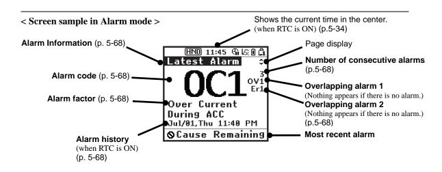
Figure 5.12 Screen Samples In Running and Alarm Modes
