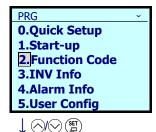
2. Use the  $\bigcirc / \bigcirc$  keys to select [2. Function Code], and confirm with the (st) key.
