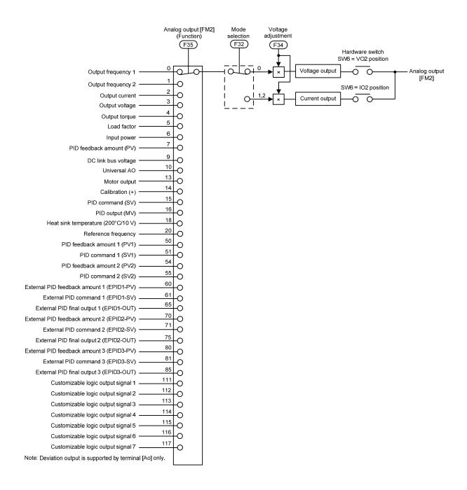
Figure 7.7 Terminal [FM2] Output Selector
