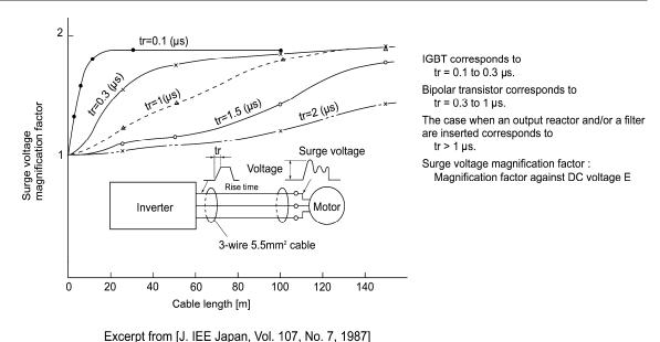
Figure B.2 Measured Example of Wiring Length and Peak Value of Motor Terminal Voltage
