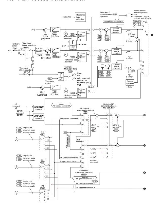
Figure 7.4 (1) PID Process Control Block
