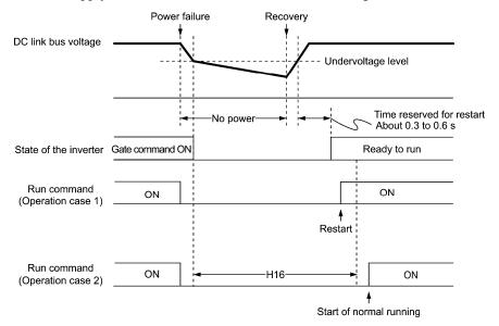
If H16 (Allowable momentary power failure time) is set to "Auto," restart will take place until the DC link bus voltage drops down to the allowable voltage (100 V) for restart after a momentary power failure. If the DC link bus voltage drops below the allowable voltage, the inverter recognizes that the power has been shut down so that the inverter does not apply the restart mode and starts normal running.
