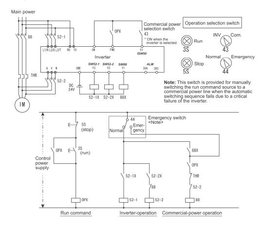
3) Sequence with an emergency switching function -- Part 2 (Automatic switching by the alarm output issued by the inverter)
