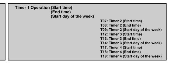
These function codes specify the start time, end time, and start day of the week for timer operation; T02 to T4 for Timer 1, T07 to T09 for Timer 2, T12 to T14 for Timer 3, and T17 to T19 for Timer 4.
