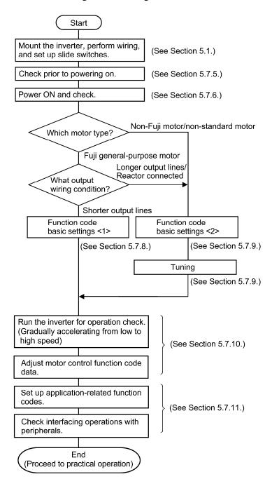
Figure 5.16 Test Run Procedure
