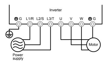
Figure 5.17 Connection of Main Circuit Terminals
