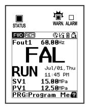
Fig. 9.1 Light alarm display example
