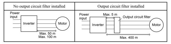
For an inverter with an output circuit filter installed, the total secondary wiring length should be 400 m or less.
