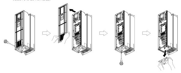
Figure 5.2 Removing the Front Cover and the Wiring Plate (FRN37AQ1M-4□)
