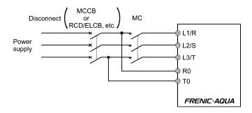
7. Install UL certified fuses or circuit breaker between the power supply and the inverter, referring to the table below.
