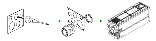
Figure 5.3 Punching Out Semi-perforated Sections in the Wiring Plate and Setting Cable Glands or Conduits
