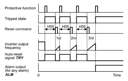
The auto-reset operation can be monitored from the external equipment by assigning the digital output signal TRY to any of the programmable, output terminals [Y1] to [Y4], [Y5A/C], and [30A/B/C] with any of E20 through E24 and E27 (data = 26).
