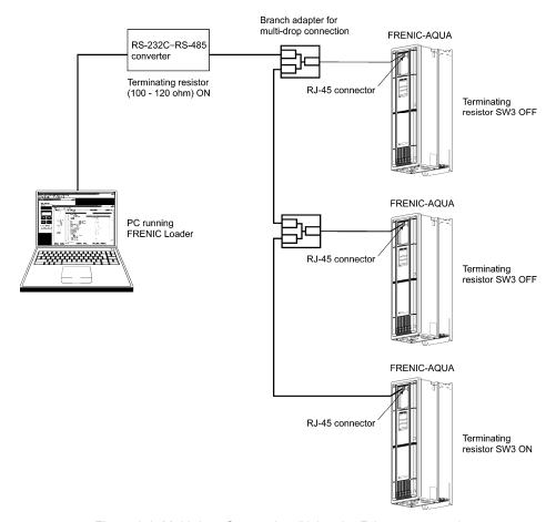
Figure 8.1 Multi-drop Connection (Using the RJ-45 connector)
