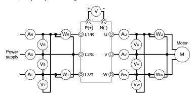
Figure 10.1 Connection of Meters
