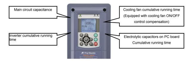
• Life warning signal can be output to transistor output.
