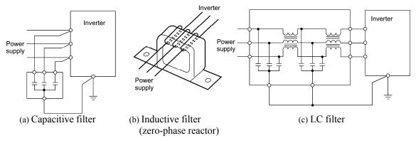
Figure A.10 Various Filters and their Connection
