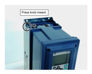
Remove the cooling fan (with case).
