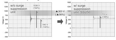
Motor/inverter capacity: 75 kW
