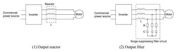
Figure B.3 Method to Suppress Surge Voltage
