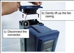
(3) Remove the cooling fan from its casing. See d).
