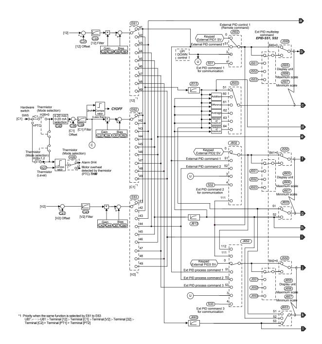
Figure 7.5 (1) External PID Process Control Block
