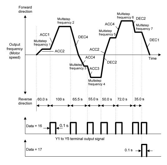
To start or stop a pattern operation, use the  $\frac{1}{2}$  keys on the keypad or turn the related input terminals ON/OFF.
