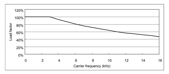
Figure 2.12 Current Derating by Carrier Frequency (Surrounding temperature: 50°C for IP21, 40°C for IP55)
