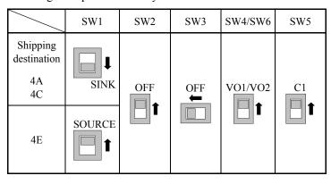
Figure 5.5 Location of the Slide Switches on the Control PCB
