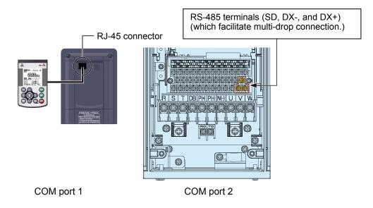
Using the RS-485 communications ports shown above enables the extended functions listed below.
