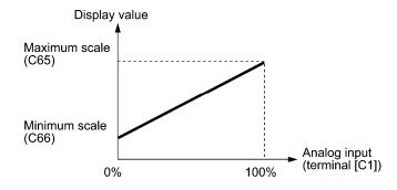
Example: To detect 0 to 30 kPa with 4 to 20 mA output of the pressure sensor
