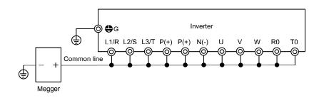
Figure 10.2 Main Circuit Terminal Connection for Megger Test
