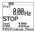
Figure 5.18 Display of the LCD Monitor after Power-on
