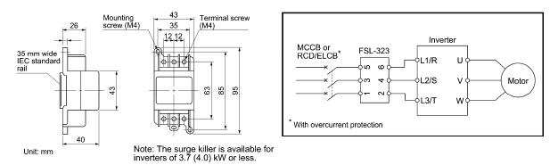
Figure 4.3 Dimensions of Surge Killer and Connection Example
