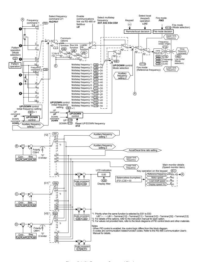
Figure 7.1 (2) Frequency Command Block
