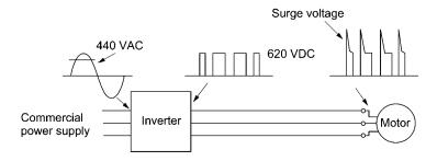
Figure B.1 Voltage Waveform of Individual Portions
