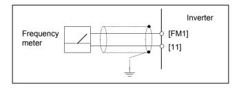
Figure 4.10 Frequency Meter Dimensions and Connection Example
