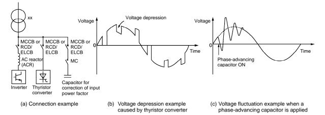
• Use an ACR when the interphase voltage unbalance ratio of the inverter power supply exceeds 2%.
