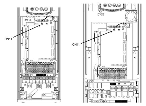
Figure 4.13 Battery Loaded (7.5 kW or below)
