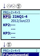
5. Use the ⊘/ ∨ keys to select the location, KP1–KP3, to store the data to be confirmed, and confirm the destination with the ⟨ key key key.
