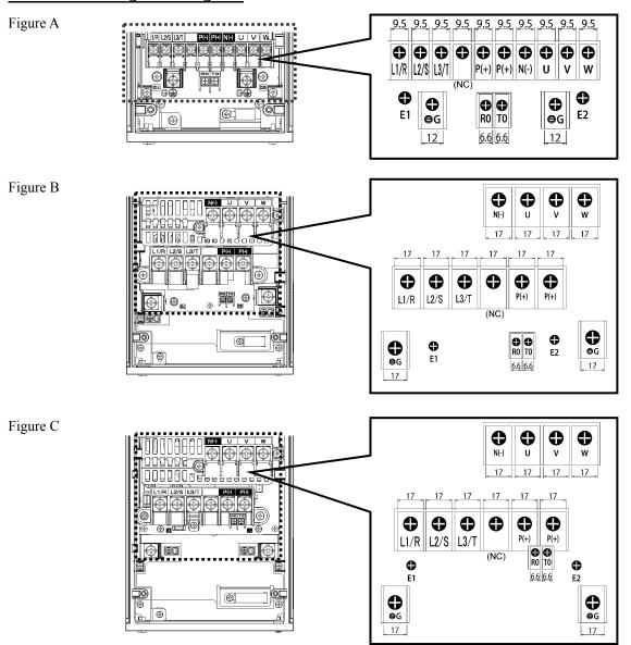
(NC): No connection (Do not make wiring.)
