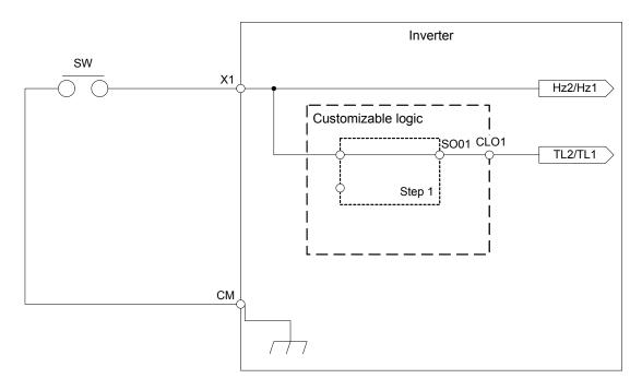
To configure the above customizable logic, set function codes as listed below. The "Type of timer" and "Time setting" require no modification unless otherwise specified.
